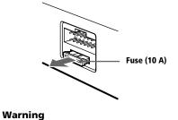
Never use a fuse with an amperage rating exceeding the one supplied with the unit as this could damage the unit.
